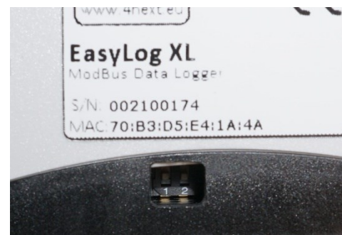
Fig. 6 Example of the DIP position: OFF
