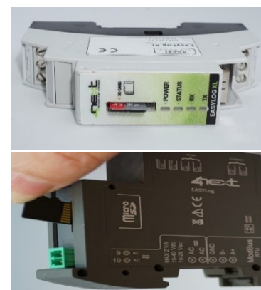
Fig. 1 SD Card Insertion EasylogXL (Top) EasyLogXL-A (Bottom)
