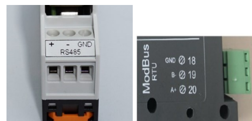
Fig. 2 RS485 connector EasylogXL (Left) EasyLogXL-A (Right)
