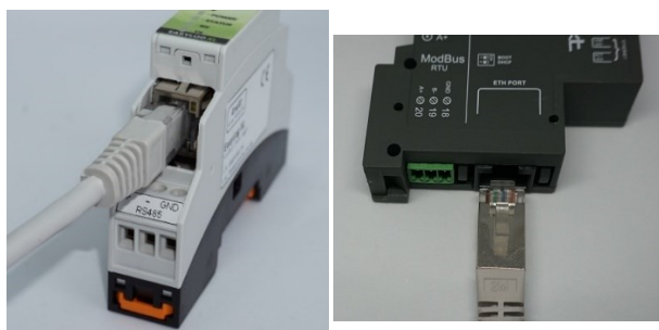
Fig. 3 Ethernet connector EasylogXL (Left) EasyLogXL-A (Right)
