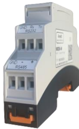
Fig.2 RS232 and RS485 serial connection
